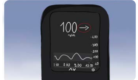
Next to the value there is a trend arrow showing how your blood glucose is changing and below it there can be a graph showing the blood glucose trend in the previous hours.
